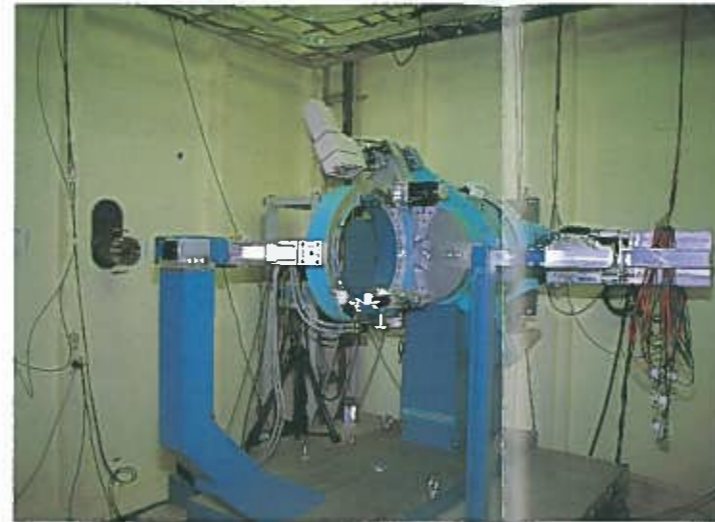
▼Protruding from the hole in the wall is the tip of a beamline. Normally, an experimental station would be installed here. (The photograph shows a measurement instrument for testing and adjusting radiant beams.)
