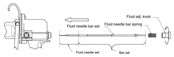
**Job-2** Screw lightly fluid needle packing set with special screwdriver and tighten further by about 30° after screw stops.
