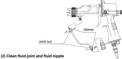
Wipe off paint stuck on fluid joint and fluid nipple by attached cleaning brush.
