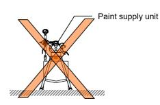
**6** When painting low resistance paints and metallic paints with electrostatic spray gun E-M10C series and using more than 2 guns at the same site, separate individual paint supply unit. If you try to use 2 guns with one set of paint supply unit and charge one gun only, the other gun, which is not charged, can be charged through paint. Then, paint and solvent can catch fire.
