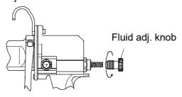
Job-2 Pull out fluid needle spring and fluid needle bar set.
