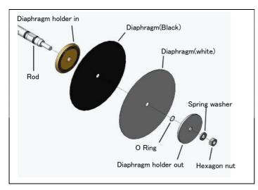
Job 2 Remove the following parts beginning with the rod from the side where hex. nut is removed:
