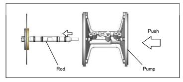
While pushing the rod from the side where hex.nut is removed, hold diaphragm where hex. nut is not removed and pull rod from main body.
