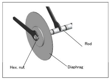
Job 4 Hold center of rod, remove hex.nut and remove following parts beginning with the rod.
