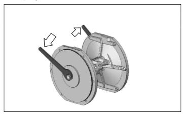
Job 1 Loosen hex. nuts which are on both sides of diaphragm. You can remove either one of them.
