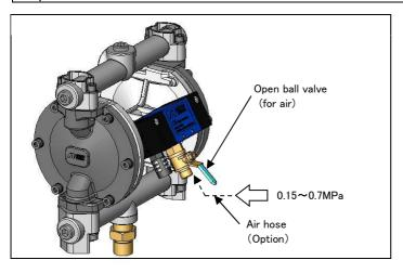
Please open the ball valve (for air) to operate pump.
