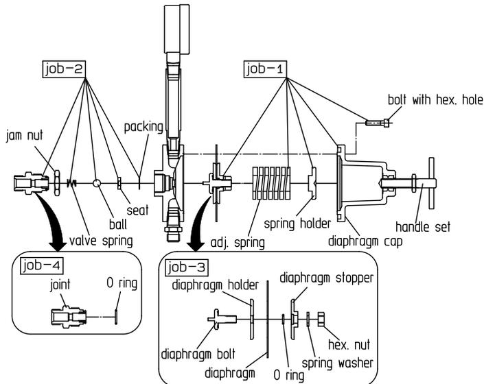
**Job-1** Fully loosen handle set, and remove bolt with hex. hole, diaphragm cap, spring holder, adjusting spring and diaphragm section.
