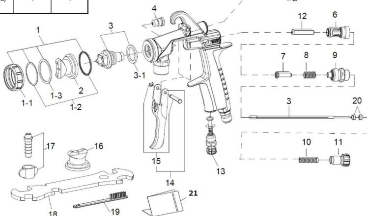
◎ When ordering parts, specify spray gun's model, part name with ref. No. and marked No. of air cap assy, fluid nozzle and fluid needle.
