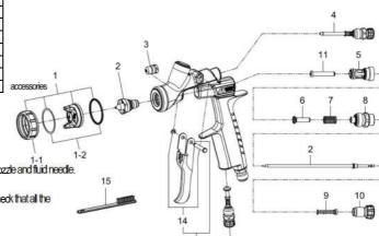
Marked parts are wearable parts.
